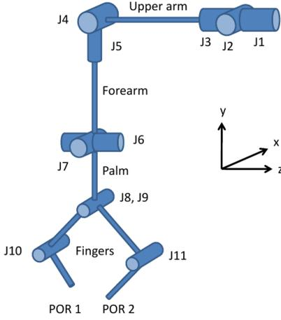
Fig. 1. The bifurcated manipulator (not drawn to scale) used in the simulations. A POR is defined at the end of each “finger.”
