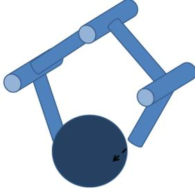
Fig. 2. The manipulation scenario. The two-finger manipulator is initially contacting the object lightly. At the start of the simulation, the right finger impedance position reference changes so that the finger will move in the direction of the dashed arrow. The left finger impedance remains unchanged so that it will continue to apply a light inward force on the object. The dual-priority control law must move the right finger without changing the impedance of the left finger.
